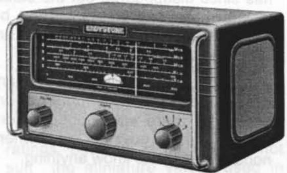
Model S.870A 'cabin set' of 1960 was Eddystone's smallest valve AC/DC radio at just 11 inches wide
